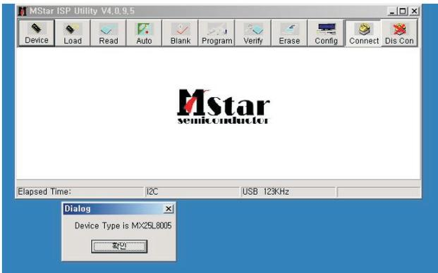
3) Click the Config button and Change speed E2PROM Device setting : over the 350KHz
